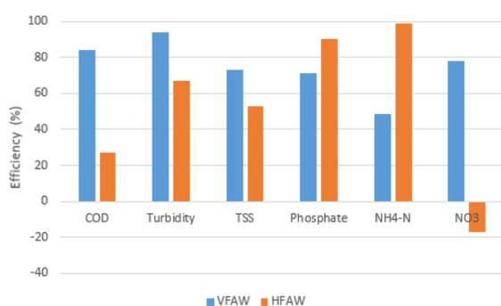
**Figure 12.** Vertical and horizontal wetland efficiency with a wastewater sample
