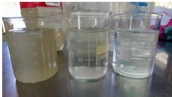
**Figure 13.** Turbidity of the treated wastewater in the hybrid system of artificial wetlands.
