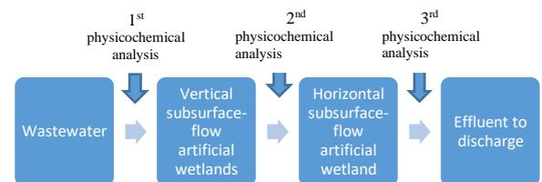
**Figure 7.** Diagram of the hybrid artificial wetland system process
