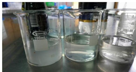
**Figure 8.** Turbidity of treated synthetic wastewater in the hybrid artificial wetland system.
