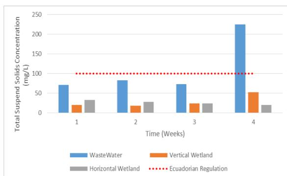
**Figure 10.** Total suspended solids concentration in the hybrid wetland system
