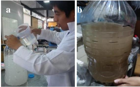
**Figure 4a.** Manufacture of synthetic wastewater
