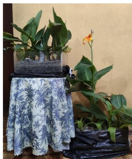
**Figure 14.** Pilot plant. Artificial hybrid wetland system after 6 weeks of experimentation
