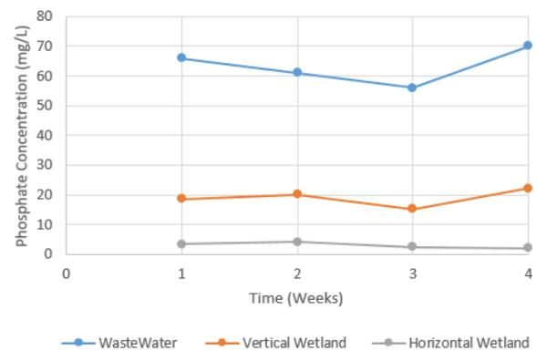
**Figure 11.**  $\text{PO}_4^{3-}$  concentration of the hybrid wetland system
